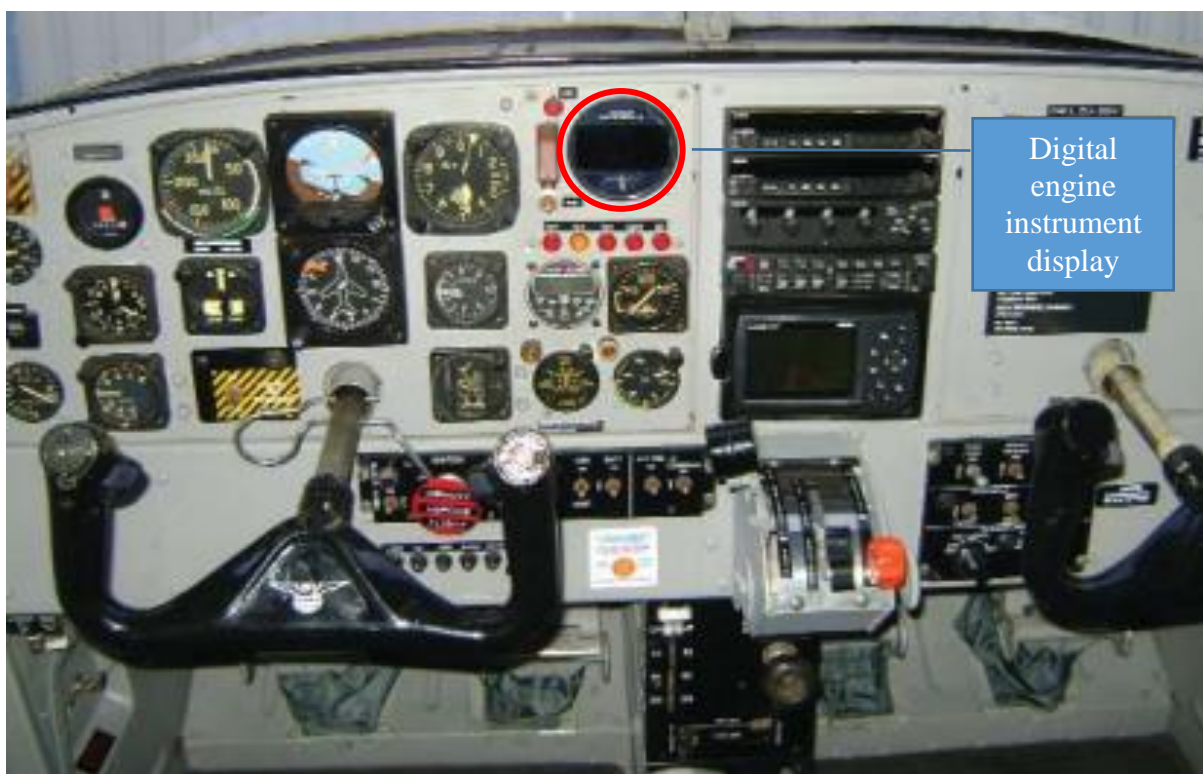
Figure 2: The cockpit layout of the Atlas Angel (World Air News November 2009, Page 8)
