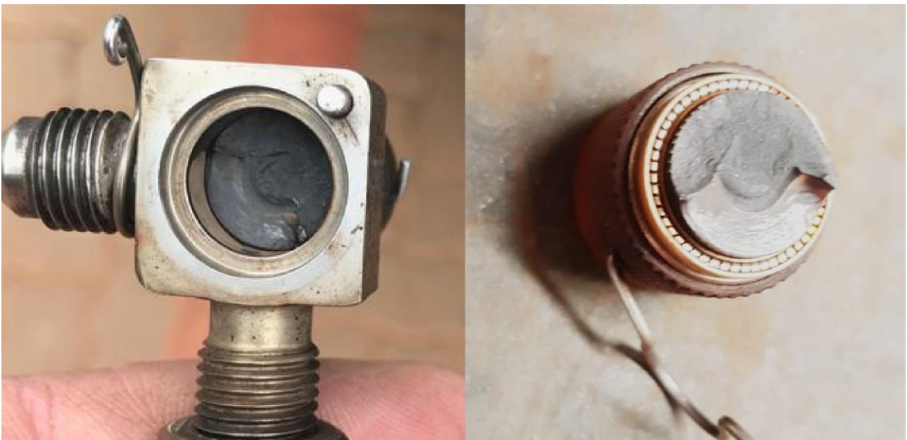
Figure 5 & 6: The Pc Safety Valve was found broken and the half stem could not be found. (Source: Approved Maintenance Organisation)
