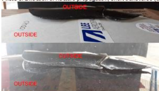
Photo 8: Comparative contouring between new (top) and used (bottom) cabin windows (digital)
