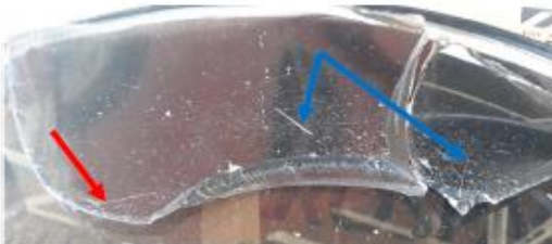
Photo 4: Remainder of cabin window showing multi-direction score marks (digital)
