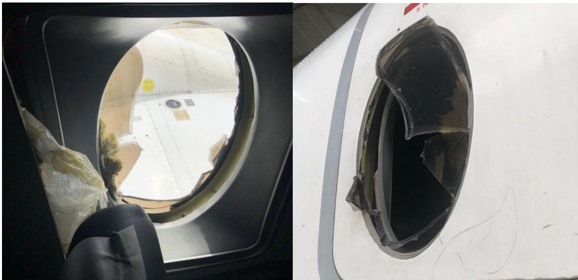
Figure 2: Internal (left) and external (right) view of the failed window
