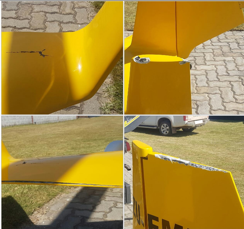
Figure 5: Damage to the rudder and tail section (Source: aircraft owner)
