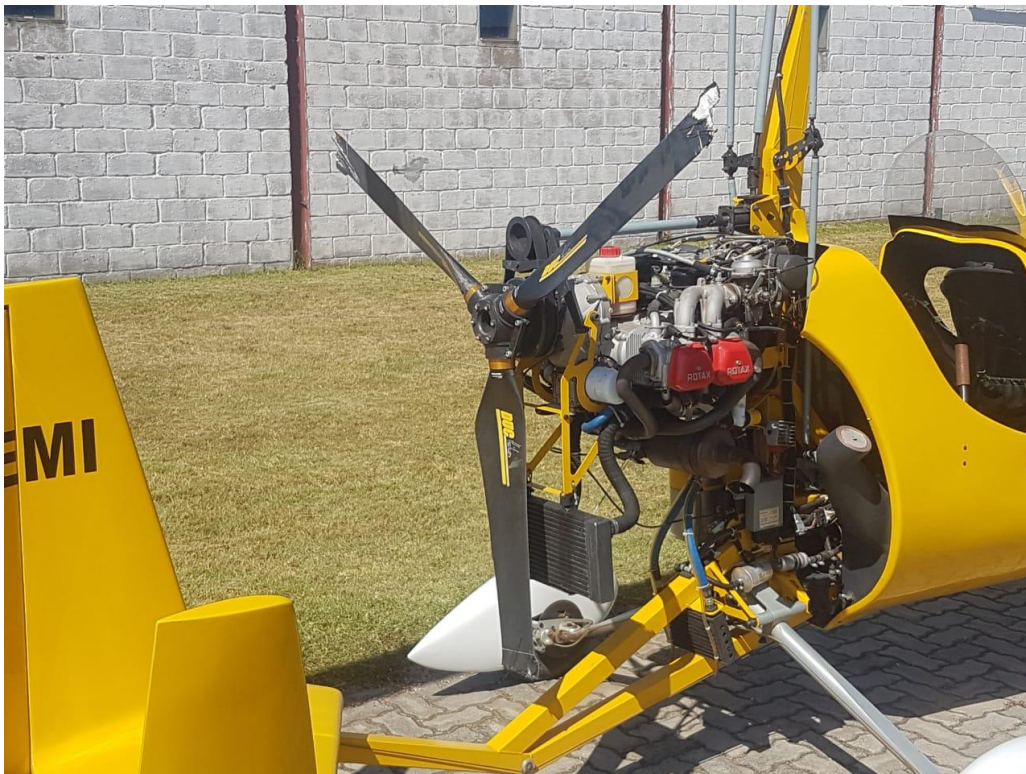
Figure 4: Damage to the propeller (Source: aircraft owner)
