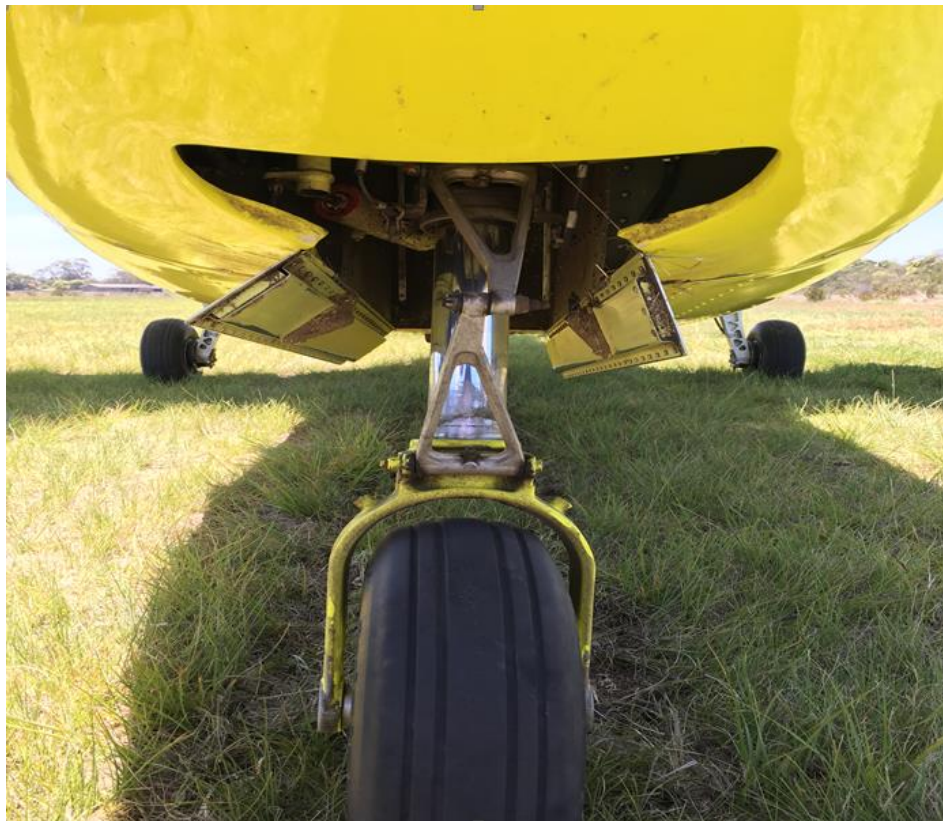
Fig. 3: Minor damage to the nose landing gear doors and rod ends (Photograph courtesy of Progress Flight Academy)
