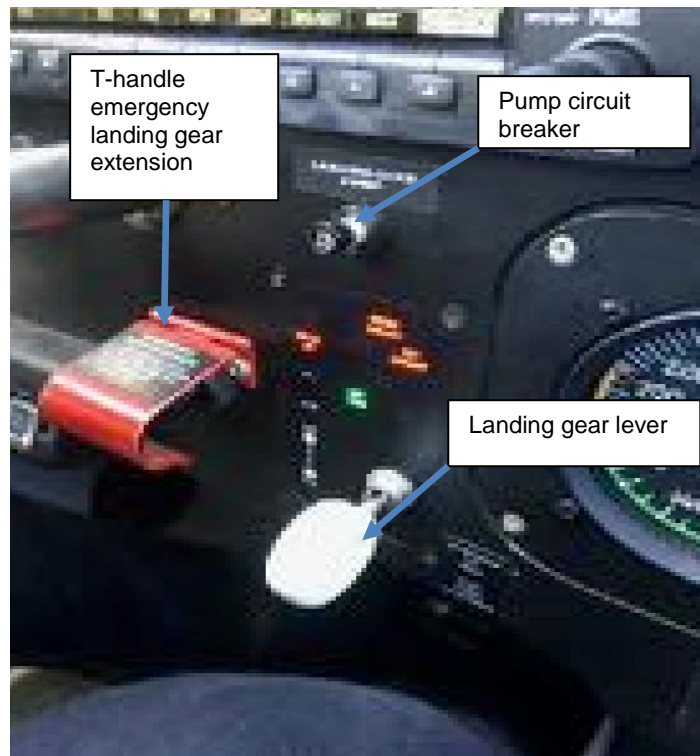
Fig. 1: Picture of the landing gear indication prior to landing (Picture courtesy of the Pilot)
