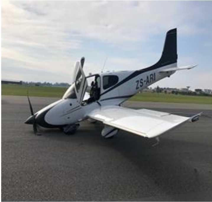
Figure 2: Damage sustained on the nose wheel.
