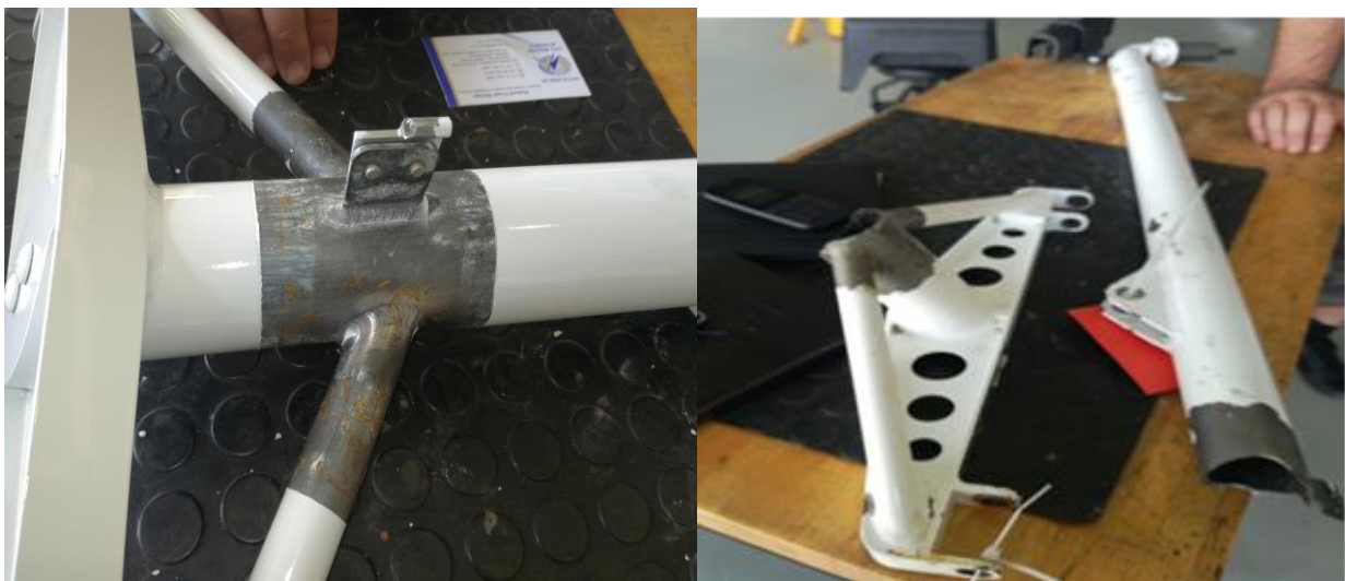
Figures 3 and 4: A failed strut tube (right) and a normal strut tube (left).
