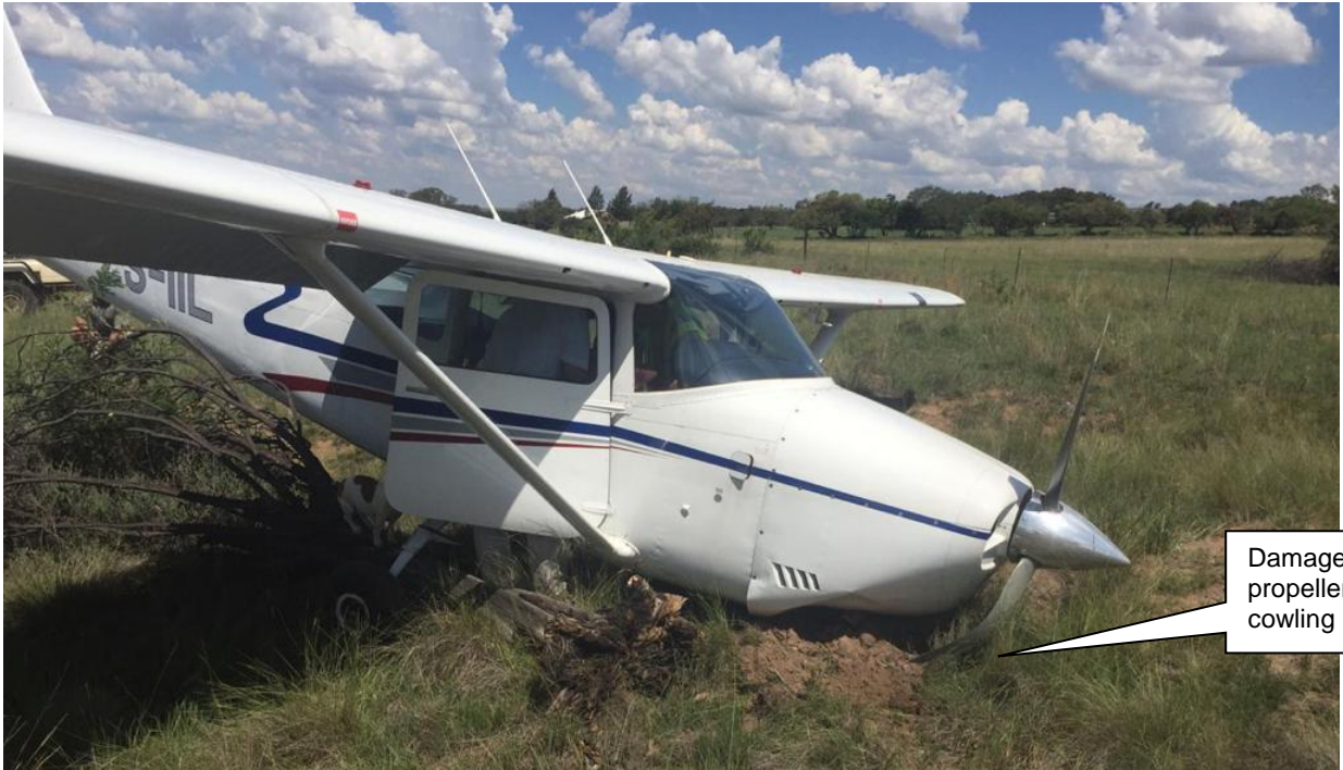
Figure 3: Damage to the propeller and cowling (Source: J de Reuck)
