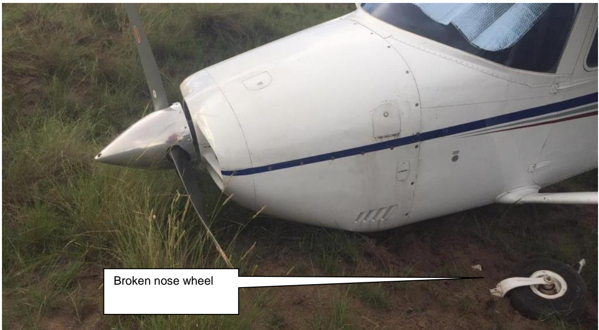
Figure 4: Damage to the nose gear (Source: J de Reuck)
