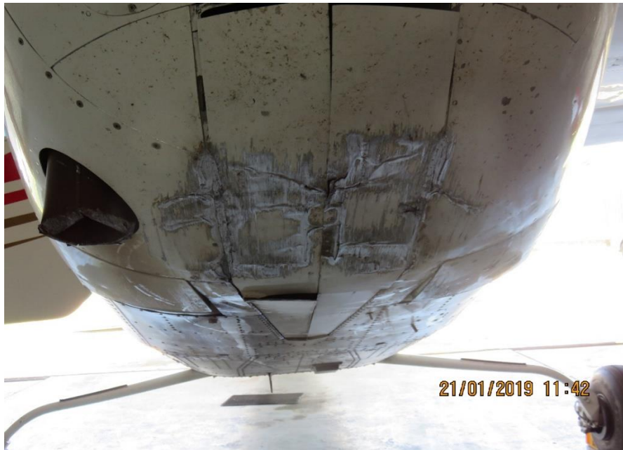
Figure 2: Damage to the nose gear doors, cowling and exhaust
