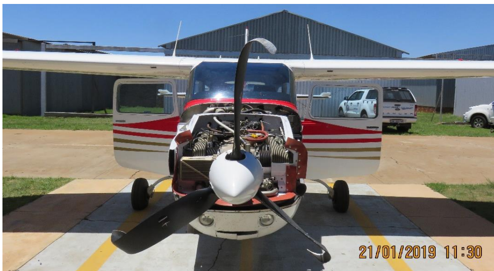
Figure 3: Damage to the propeller
