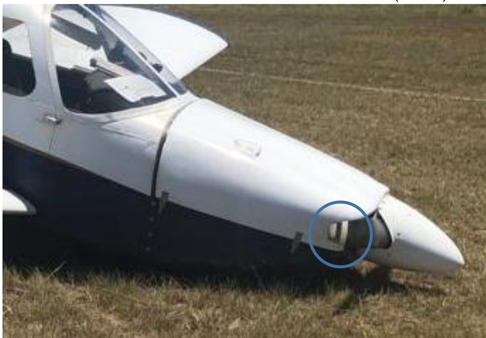
Figure 2: The damaged propeller (Source: 43 Air School)
