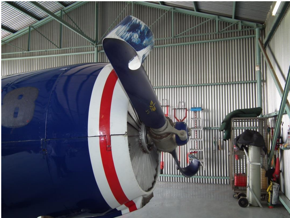
Figure 2: View of the bent propeller blades. (Photo courtesy of the pilot)
