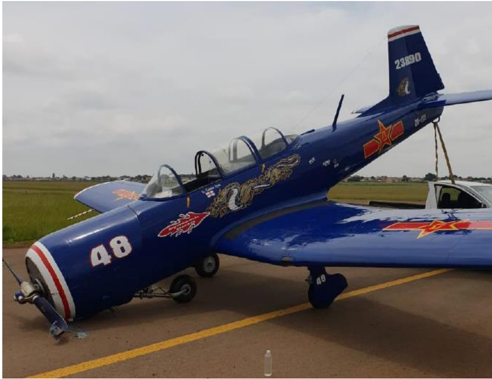
Figure 1: The aircraft after the nose gear collapsed. (Photo courtesy of the pilot)
