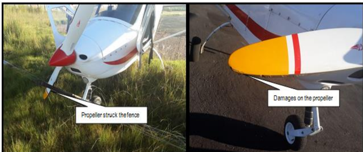
Figure 1: Damage on the propeller after the incident.
