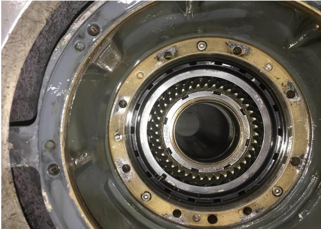
Figure 10: Two of the loose bearing house assembly bolts. (Source: Standard Aero)
