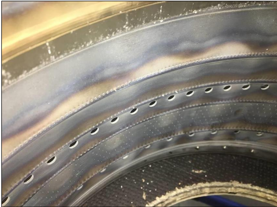
Figure 13: Debris within the cooling holes of the combustor liner. (Source: Standard Aero)
