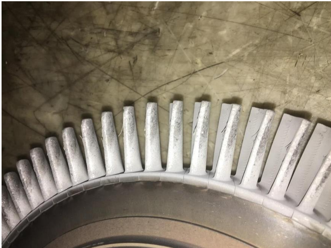
Figure 14: Metal splatter on the first turbine blades. (Source: Standard Aero)
