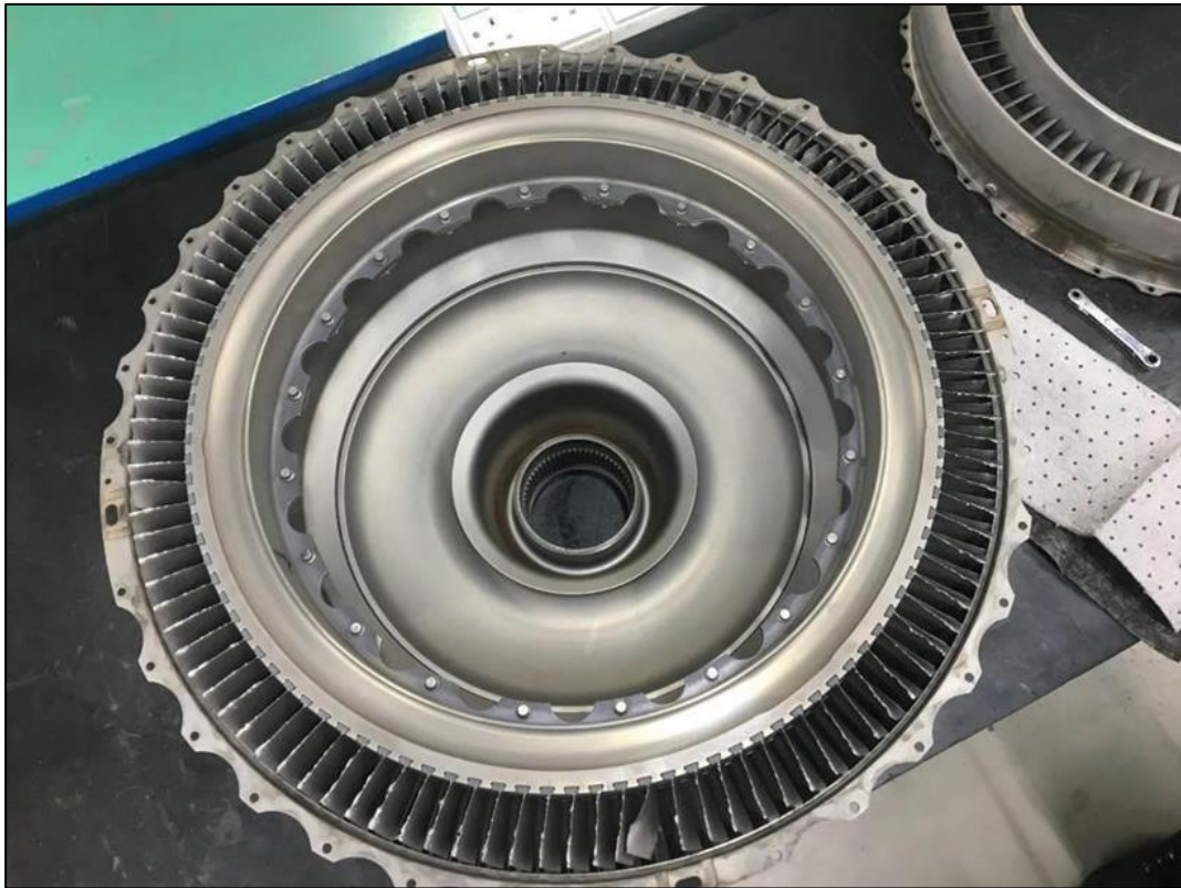
Figure 4: Impact damage to the second stage LPC blades. (Source: Standard Aero)
