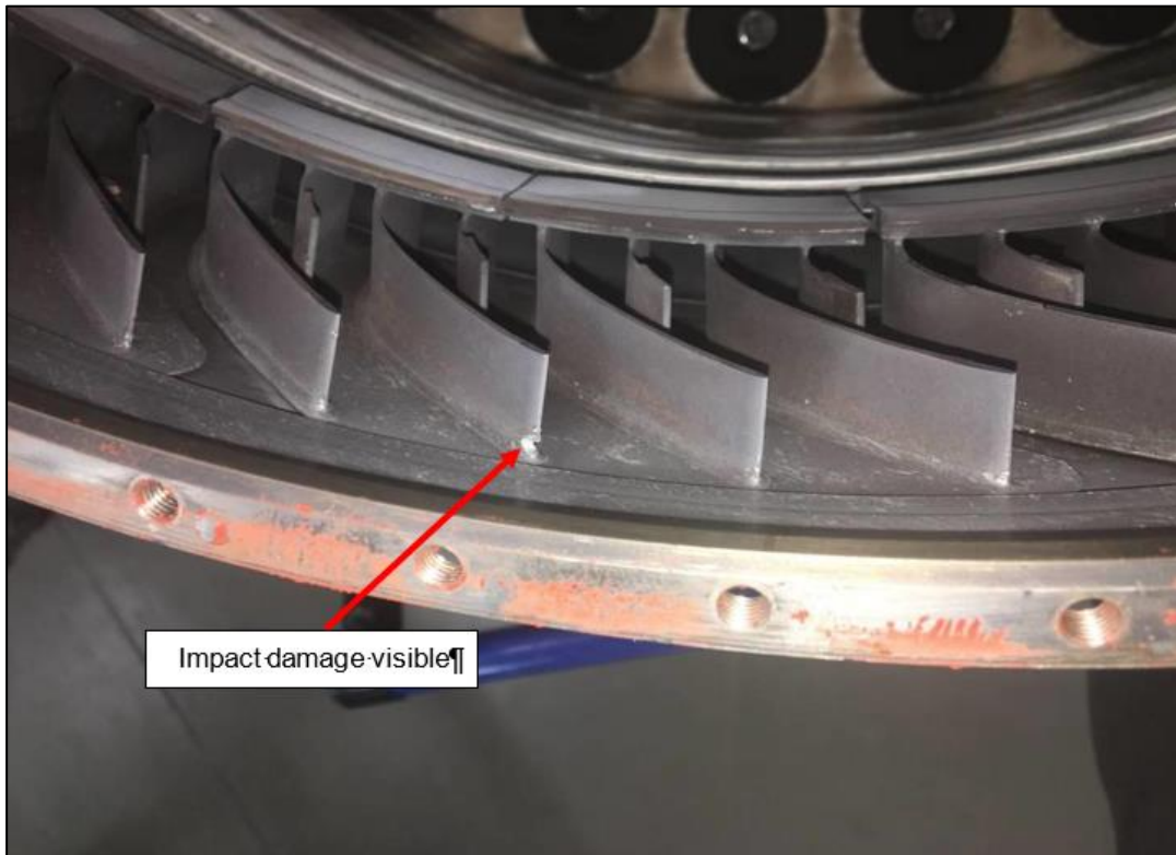
Figure 12: Impact damage to the combustor turning vanes. (Source: Standard Aero)
