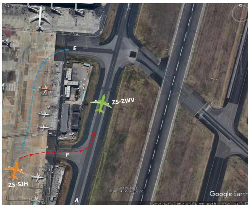
Figure 1: Blue line shows the route that was given to ZS-SJH by the GND ATC and the red line shows the route taken by ZS-SJH.
