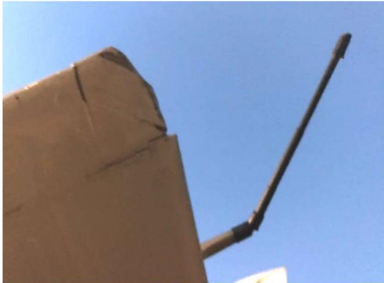
Figure 6: The damaged static wick and the left-hand horizontal stabiliser tip on ZS-ZWV. (Picture courtesy of Comair Limited)
