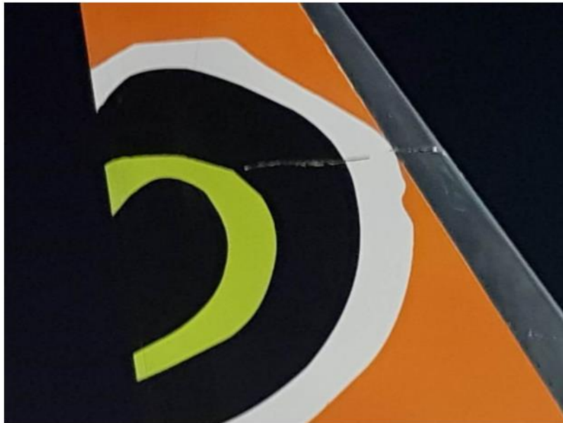
Figure 4: Picture of the damaged right-hand winglet on the ZS-SJH. (Picture courtesy of Mango Airlines)
