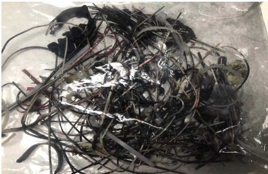
Figure 9: The wire off cuts sent to Dassault Aviation after the temporary repair was carried out. (Source: Dassault Aviation)
