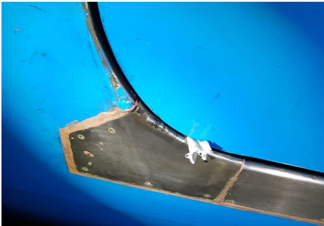
Figure 10: A section of the aft cargo door pressure seal protruding from the closed cargo door.
