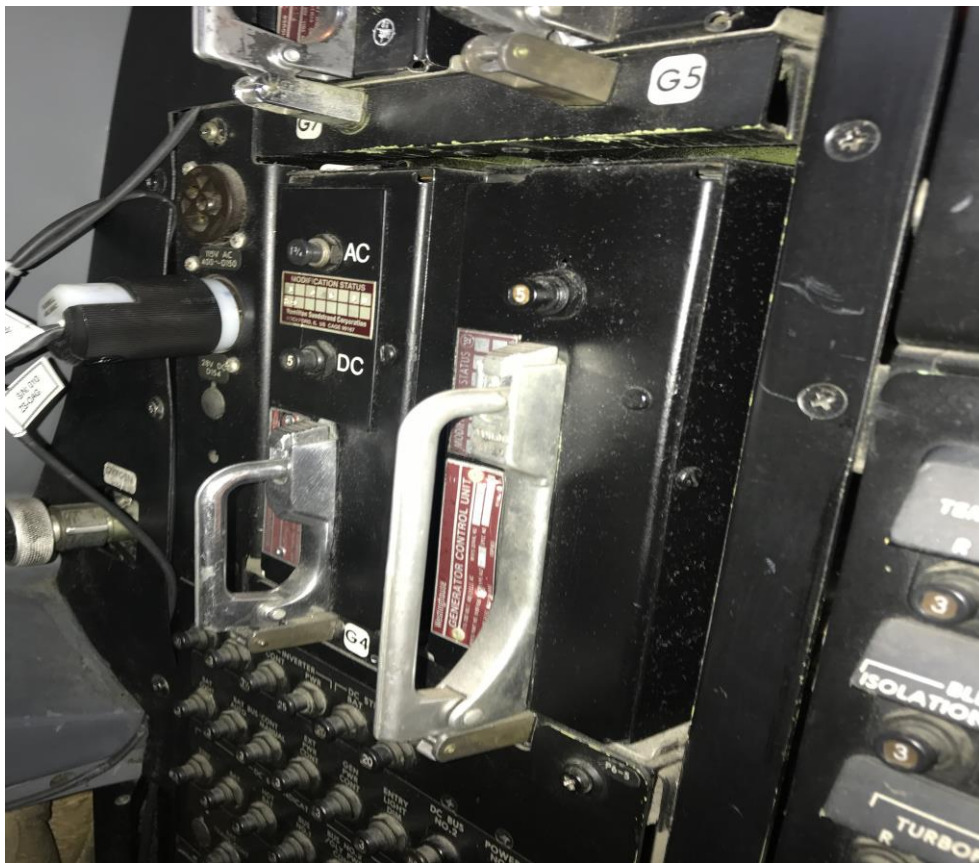
Figure 1: Generator Control Unit. (Picture courtesy of Safair)
