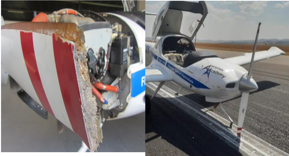
Figures 1 and 2: The damaged propeller (left) and the aircraft as it came to rest (right).
