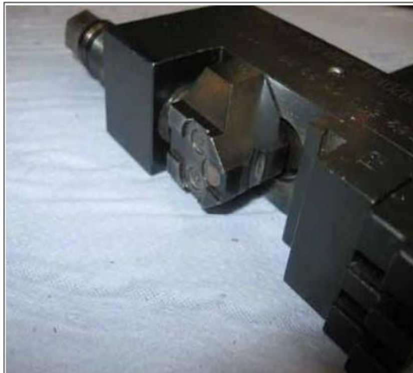
Figure 9: A special tool recommended by the manufacturer for the installation of the timing chain.
