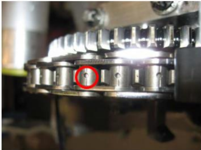
Figure 2: Original assembly of the time chain, holes in the bushings visible
