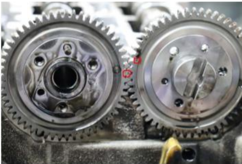
Figure 4: Synchronization of the cam shaft drive gears; shift 2 gears clockwise (~13°)
