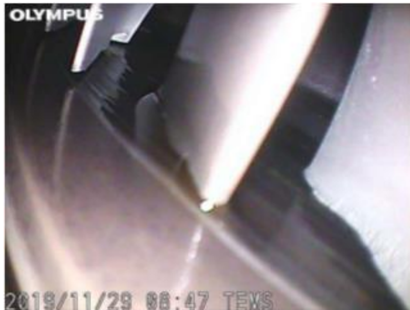
Figure 3: The HPC / impeller blade with evidence of oil on it.
