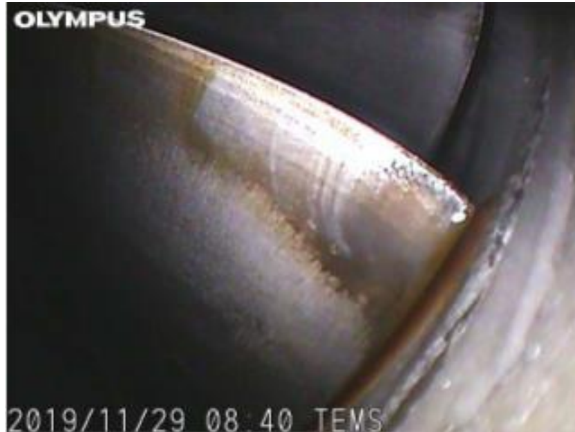
Figure 2: The high-pressure compressor (HPC) / impeller blade with oil on it.
