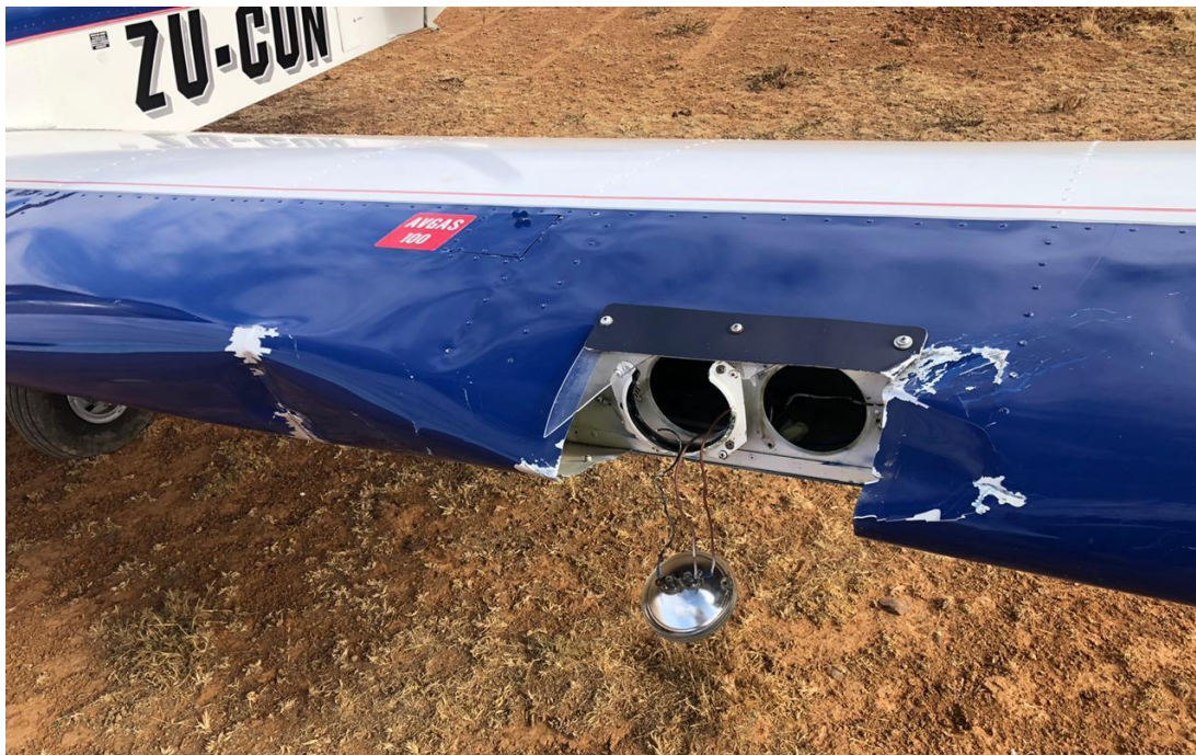
Figure 2: Damage to the left wing caused by impact with a fence post. (Photograph was taken on-site by the pilot)
