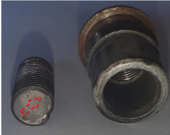
Photo 7: Locating Bush and Bolt Fracture surface (digital)
