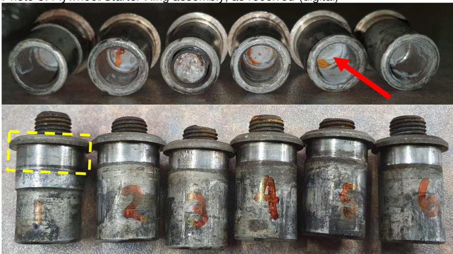
Photo 4: DriveBushes, surface conditions and geometries (digital)
