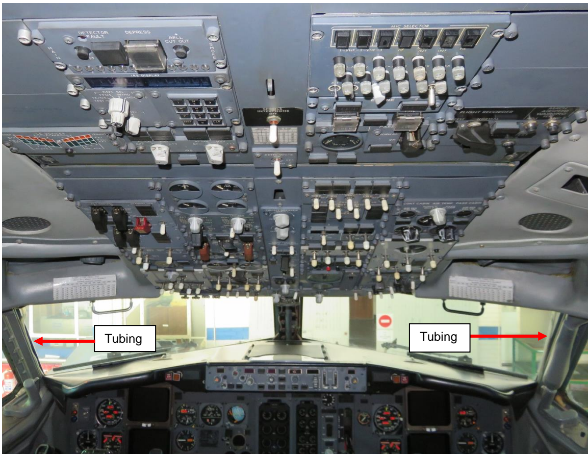
Figure 4: Cockpit of a Boeing 737-400 with the tubing (drain pipes) visible on both sides (see red arrows).
