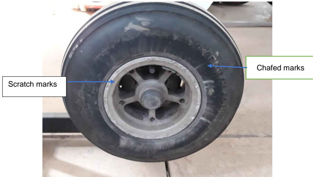
Figure 3: The aircraft tyres post-incident.
