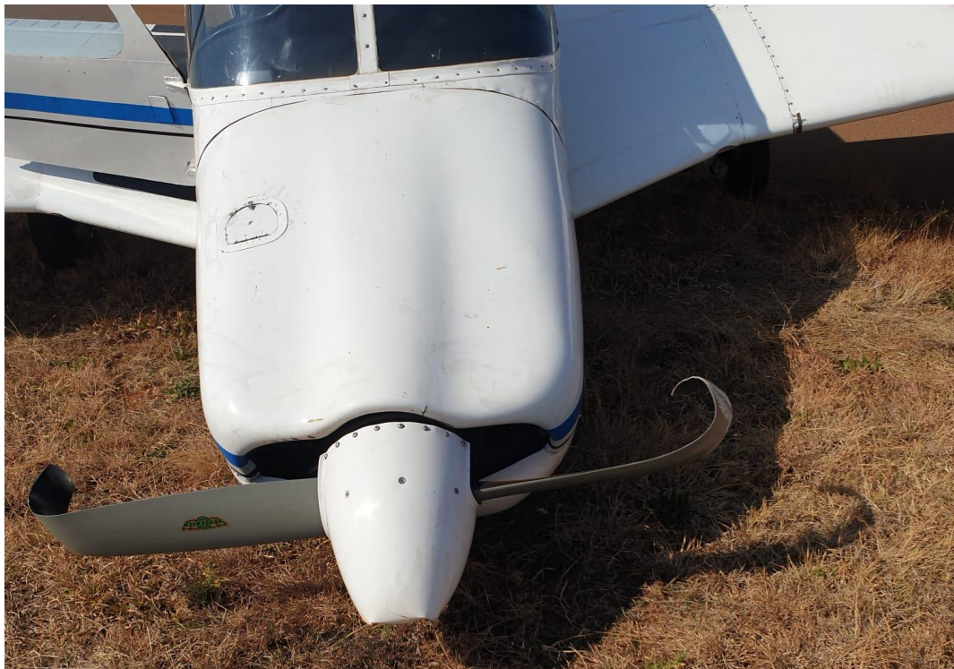
Figure 3: Both propeller blade tips were bent backwards following contact with the runway's surface.
