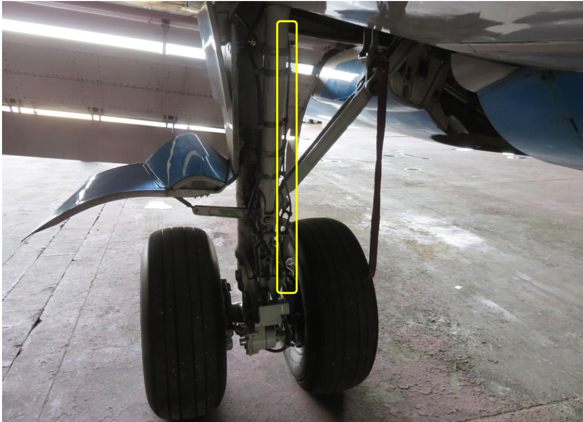
Figure 17: Right main gear (view from the front) with the Teleflex cable visible in the yellow window.
