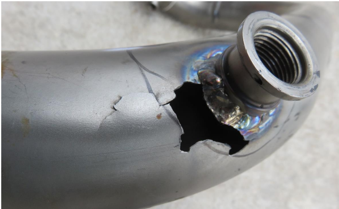
Figure 7: Damage to the aircon bay compressor outlet duct (left air-conditioning pack).
