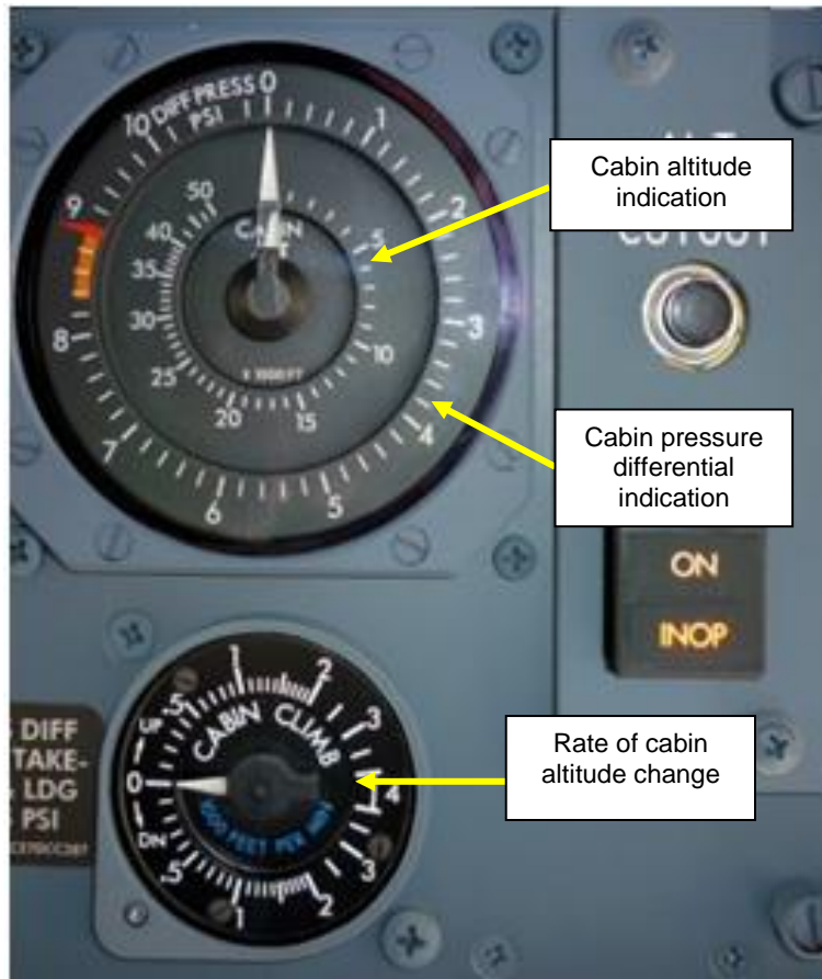
Figure 3: The visual indicators displaying the cabin altitude, the cabin pressure and the rate of cabin altitude change. (Source: B737.org.uk)
