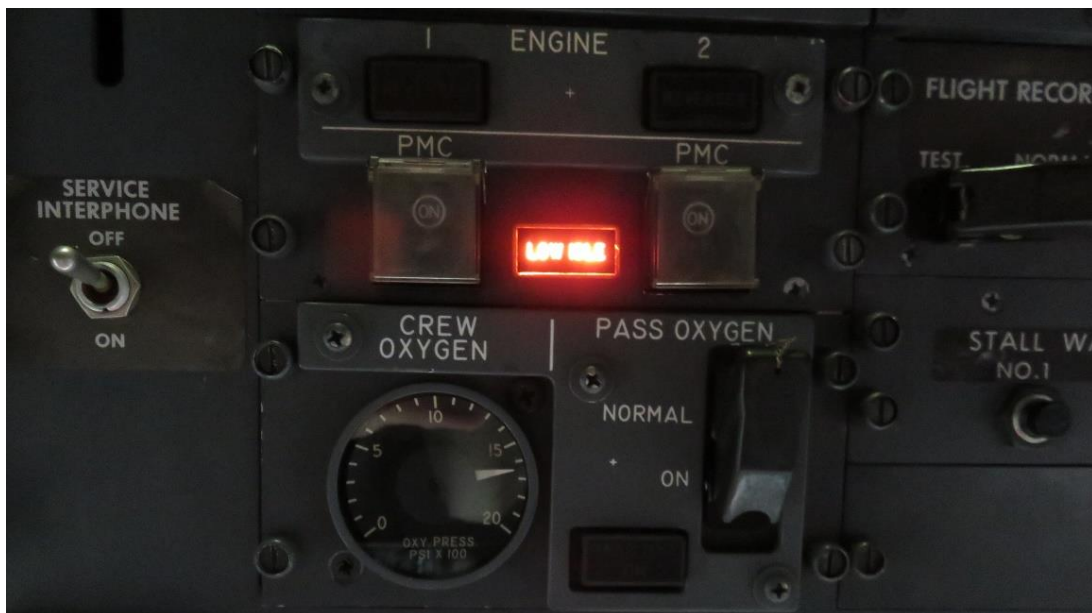
Figure 1: LOW IDLE warning for both engines, located on the overhead panel. (Aircraft in ground mode)
