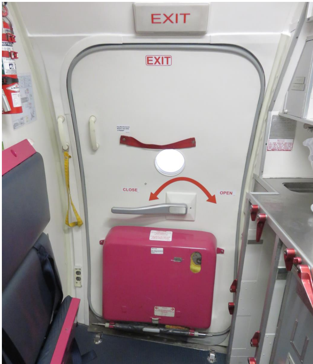
Figure 15: The right aft door (2R) in closed position.
