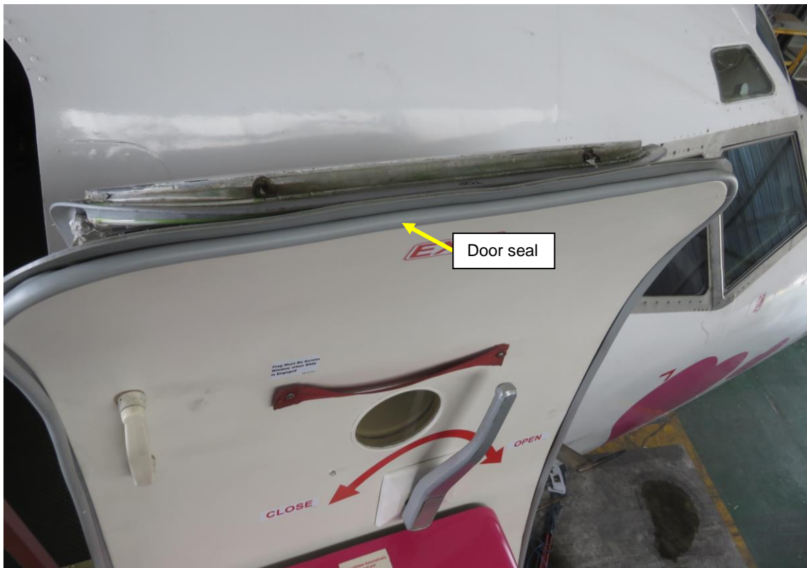
Figure 14: Door 1R in the open position, with no damage visible on the 'grey' door seal.
