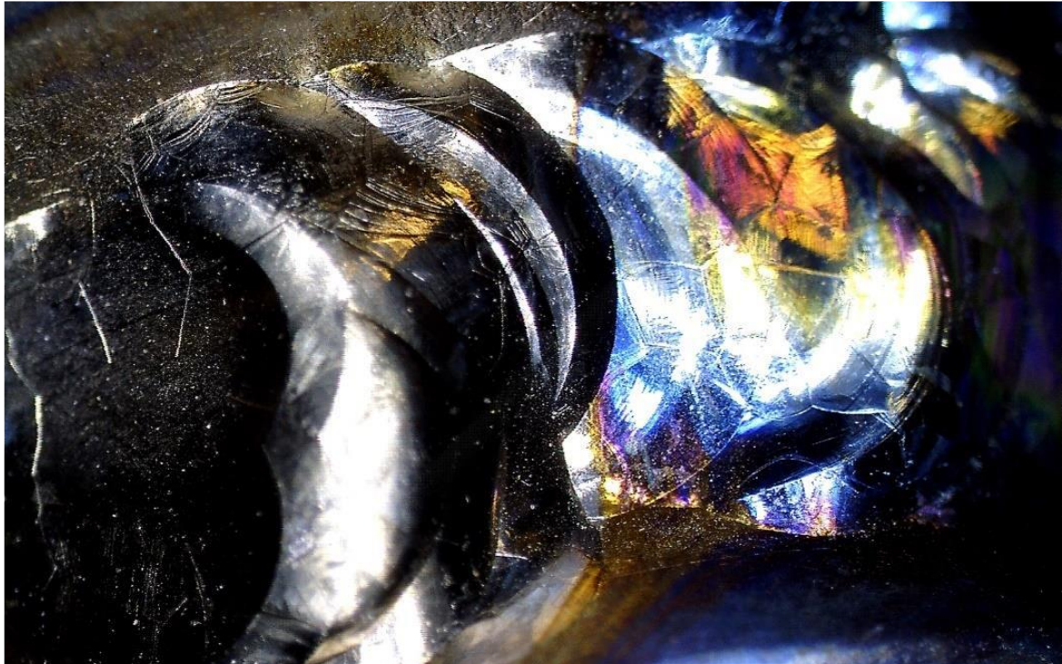
Figure 11: Magnified view of the weld surface showing the discolouration due to in-adequate shield-gas protection as well as a very irregular weld cap profile.
