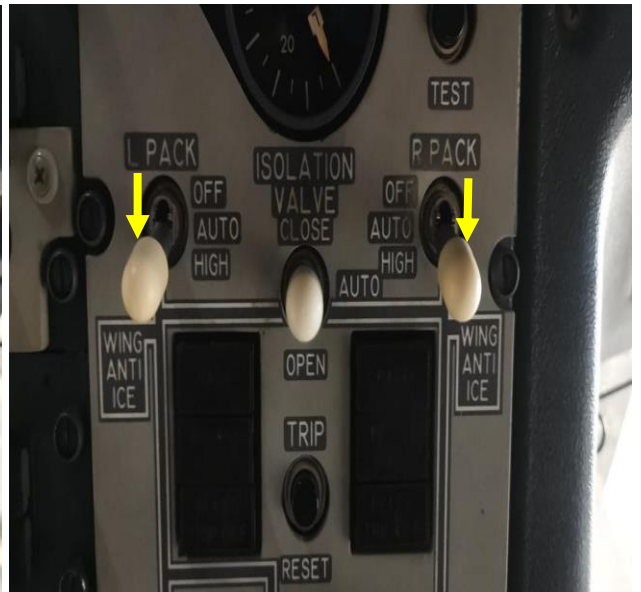
Figures 6 & 7: The aircraft pneumatic panel on the P5 cockpit overhead panel area showing the air-conditioning packs toggle switches (Bleed 1 & 2) on OFF (left) and HIGH (right).
