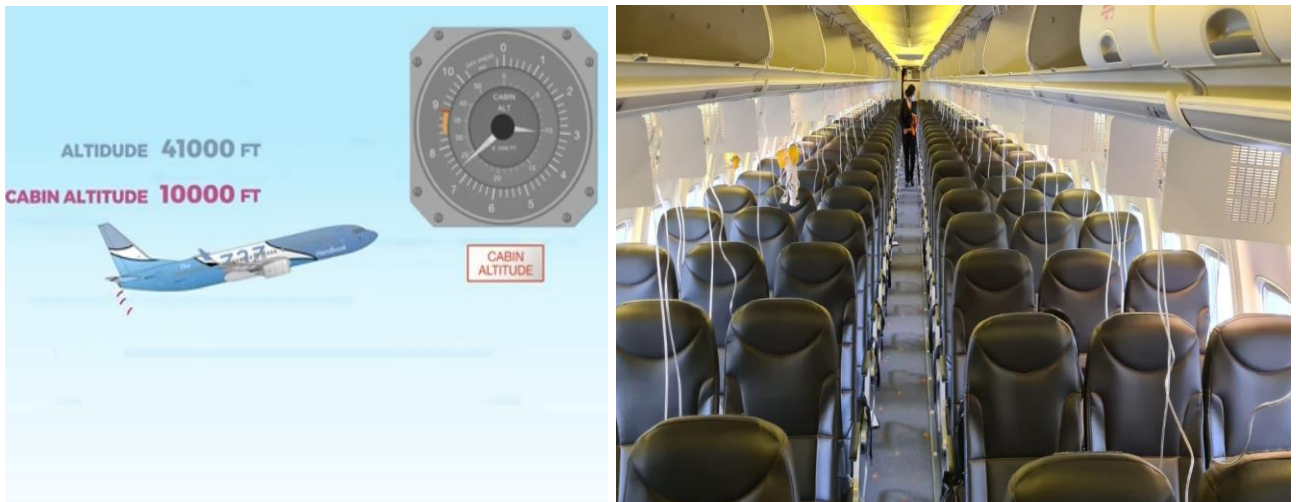
Figures 1 & 2: On the left is an illustration of a B737 aircraft animation snap shot showing the “cabin altitude” warning illuminated and the Cabin Altitude which was above 10000 ft; and on the right is a picture of the ZS-SJF aircraft showing the deployed oxygen masks.
