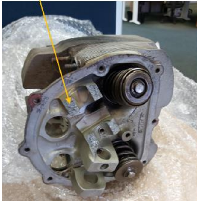
Figure 2: Damage caused to the number 5 cylinder rocker shaft boss.
