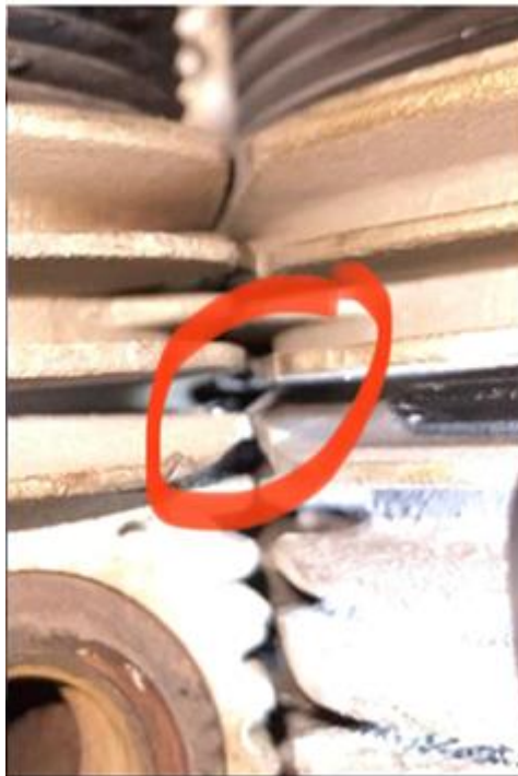
Figure 3: Hole on engine cylinder.
