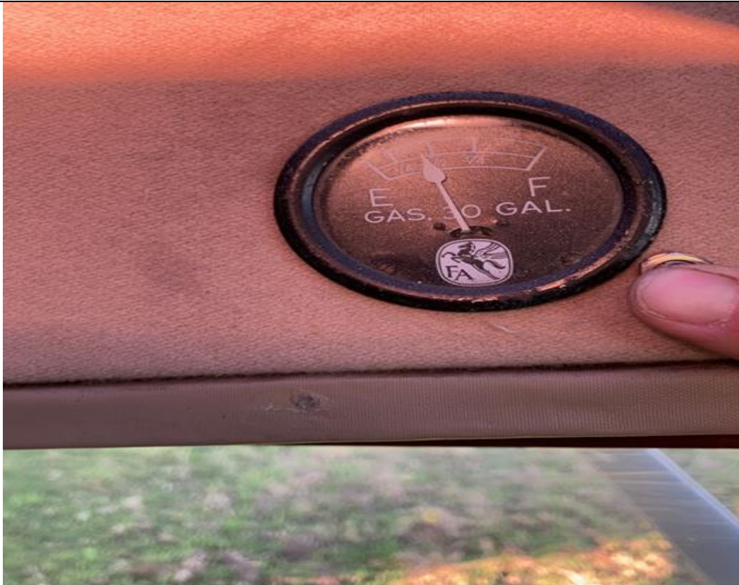
Figure 2: Gauge showing fuel remaining after the incident.
