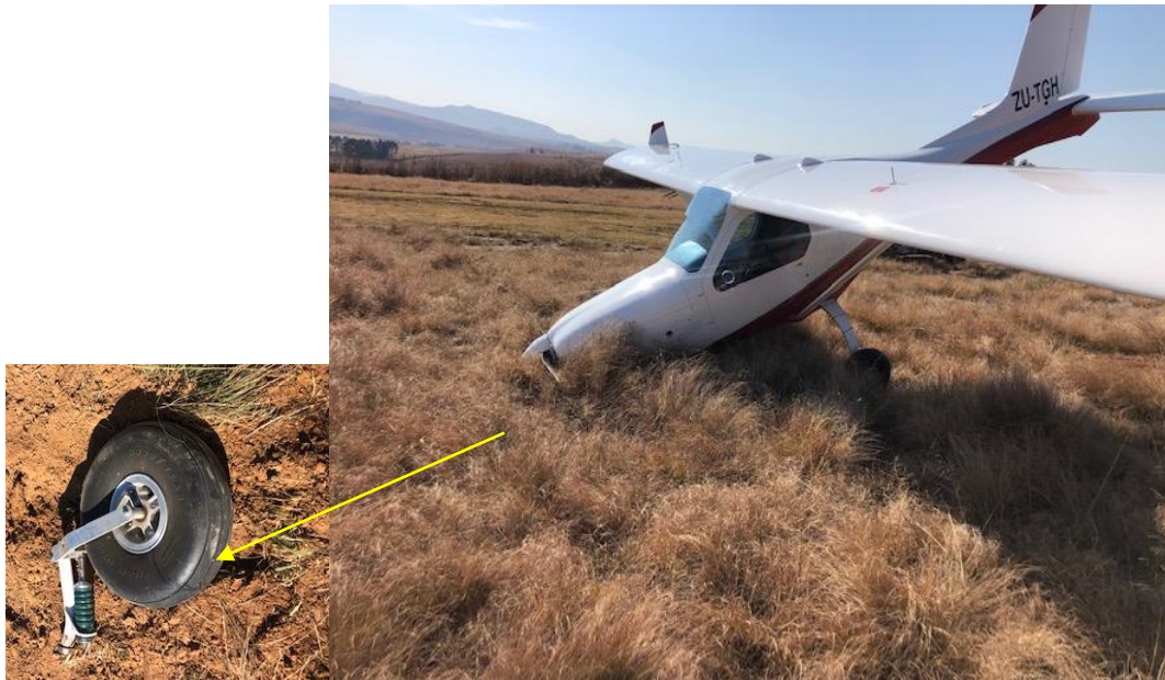
Figures 1 & 2: The final resting position of the aircraft (right picture); and a broken nose gear strut and wheel assembly (left picture). (Source: Pilot)
