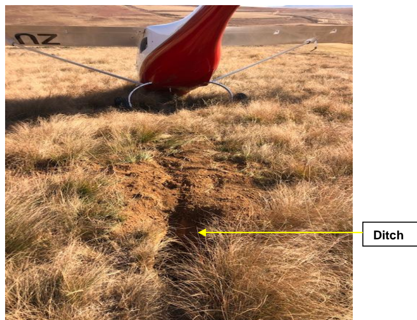
Figure 3: The rear side picture of the aircraft and the ditch that the nose wheel ran over. (Source: Pilot)
