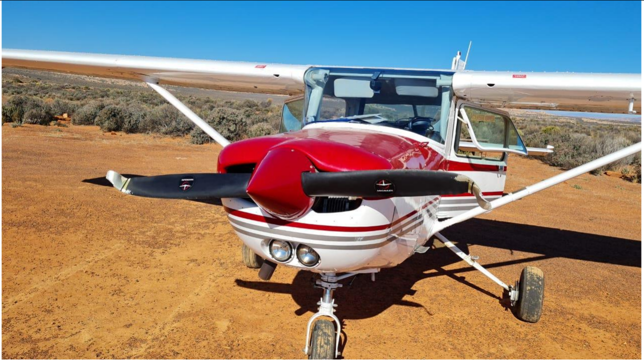
Figure 1: The aircraft at the parking bay with damage to the propeller. (Source: Pilot)
