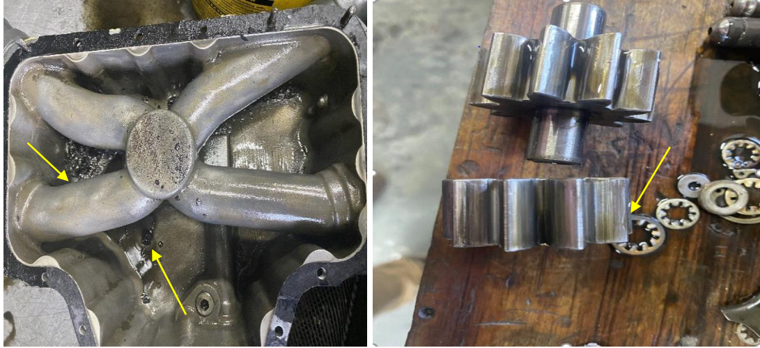
Figures 4 and 5: The oil sump indicating the presence of metal debris (left picture). The oil pump gear teeth indicating minor damage (right picture). (Source: Operator)
