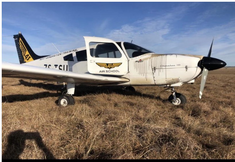
Figure 1: The aircraft at the accident site with oil streaking down the side of the engine cowling. (Source: Operator)
