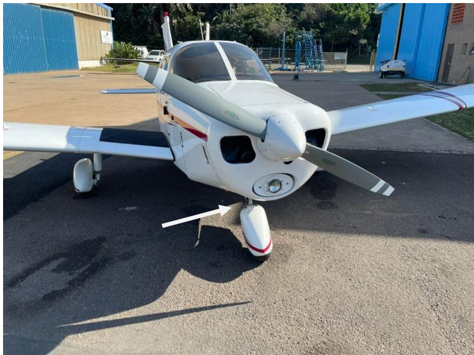
Figure 2: The nose landing gear post-accident. (Source: Approved Training Organisation)
