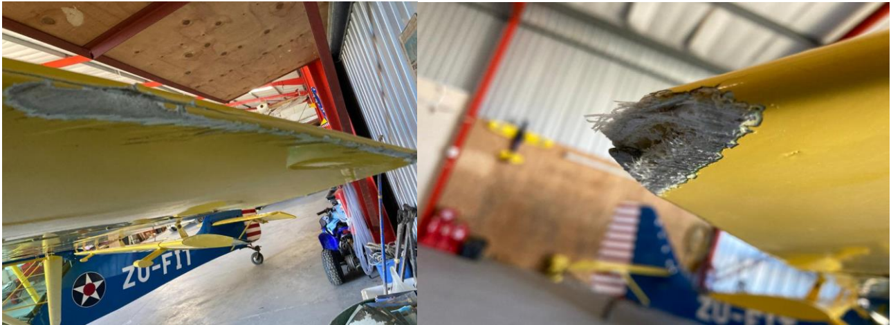
Figure 1: Scrape marks on the left-side wing tip. Figure 2: Marks on the right-side wing tip.
