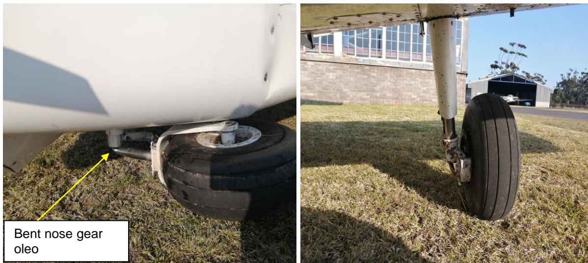
Figures 2/3: The aircraft resting on a failed nose gear strut oleo (left picture); and the condition of the left main landing gear (right picture). (Source: Operator)
