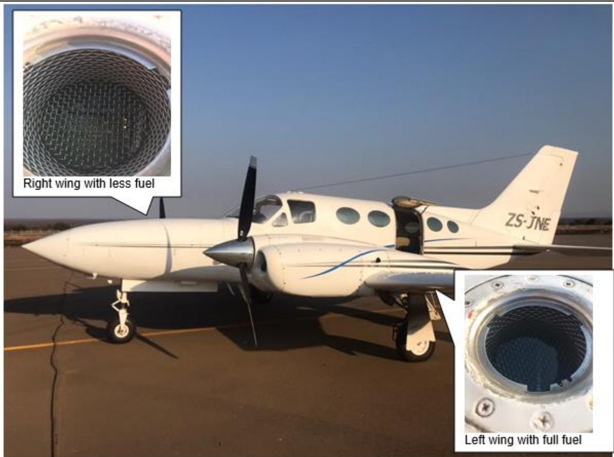
Figure 1: The aircraft post-incident with insets of right- and left-wing fuel tanks.
