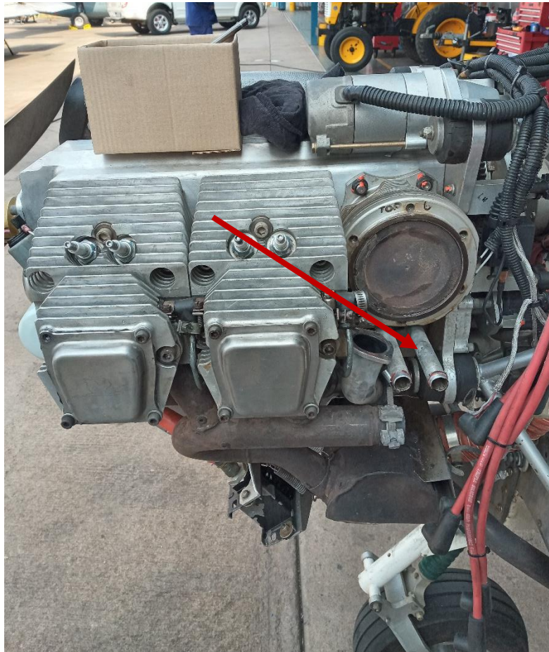
Figure 2: The number 6 cylinder out for repairs.
