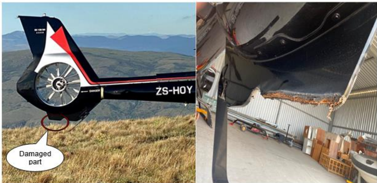
Figure 1: The helicopter fenestron damage following the incident. (Source: Pilot)
