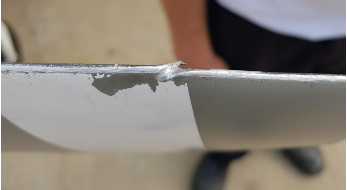
Figure 1: Indentation from the powerline on the propeller blade. (Source: ATO).
