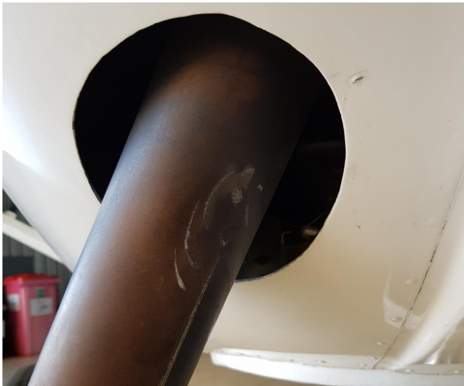
Figure 2: Wire strike markings on the exhaust.
