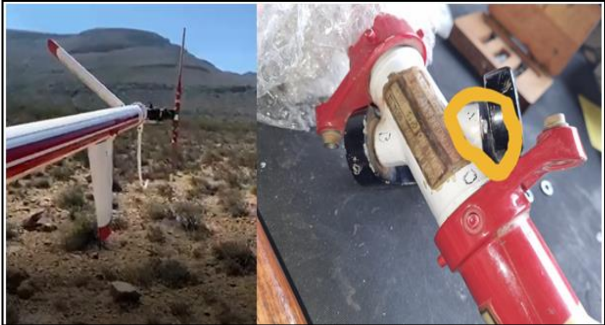
Figure 3: The aft tail boom section and the failed fork hinge bolt.
