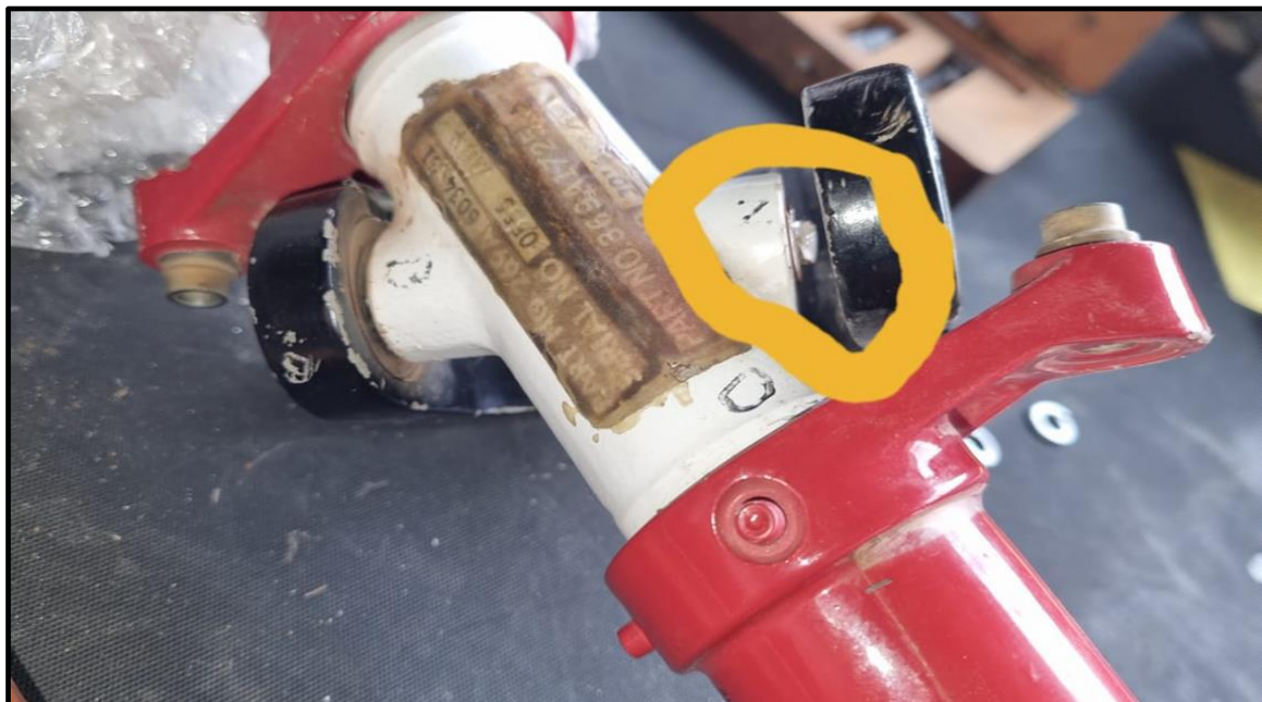
Figure 2: Damaged fork hinge bolt. (Source: Pilot)
