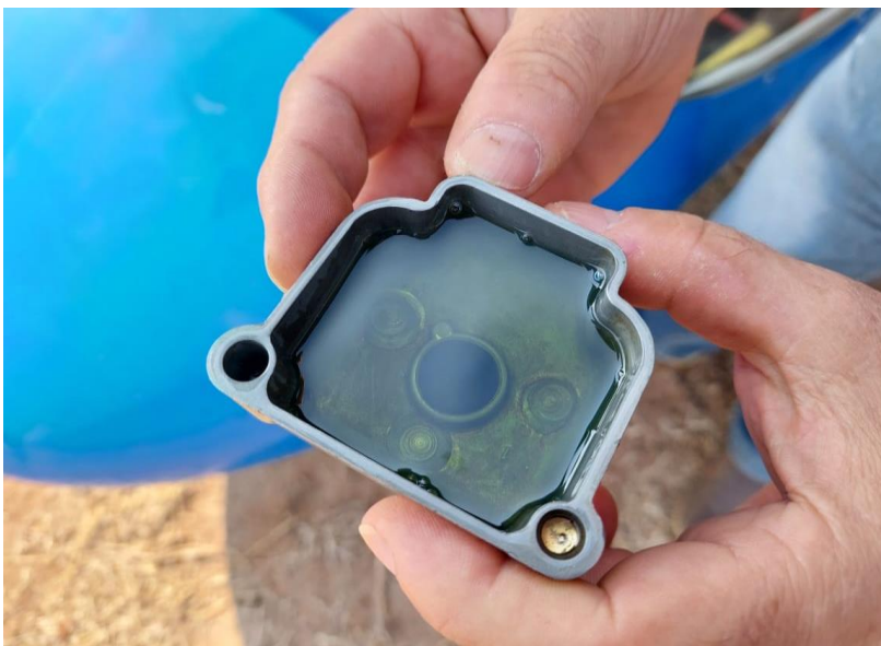
Figure 3: 95 Octane unleaded fuel found in the carburettor bowl. (Source: Operator)
