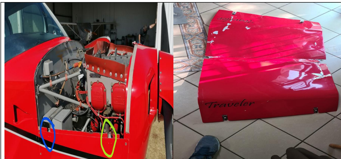
Figures 1 and 2: The engine bay and cowling cover that detached in-flight. The circle in blue indicates the starboard normal latch hook; and the circle in lime green shows the stretched hook. (Source: Pilot)
