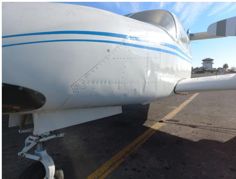
Figure 3: Wrinkles/buckles on the fuselage skin. (Source: AMO)
