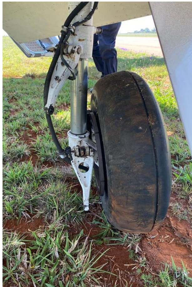
Figure 1: The left main gear torque link had separated. (Source: Pilot)
