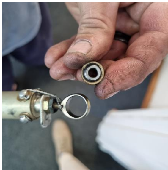
Figure 1: The rod end with the failed insert. (Source: AMO)
