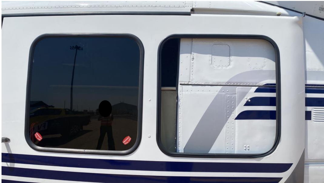
Figure 1: The left rear cargo door with no window. (Source: Operator)
