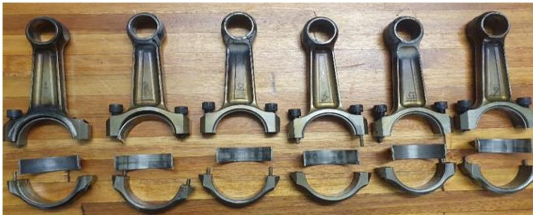
Photo 7: Conrod and BE Bearing conditions (digital).
