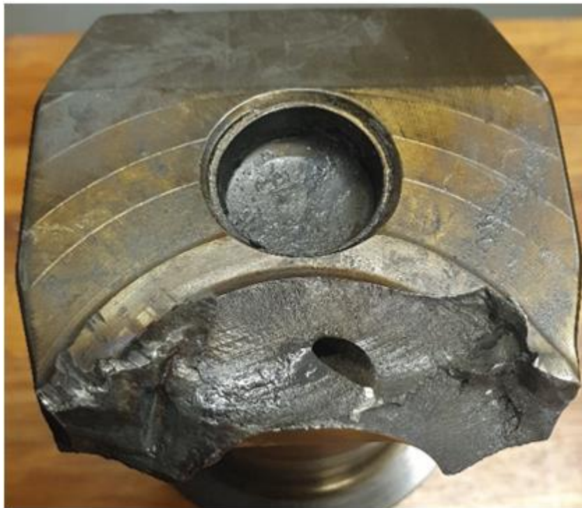
Photo 4: Fractured surface morphology (digital).
