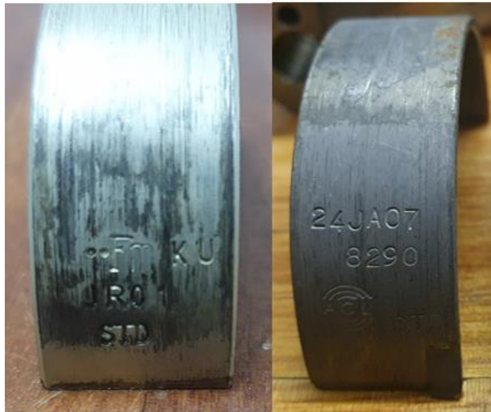
Photo 8: Variation in part numbers – Conrod BEs 2-5 (left) and Conrod BE 1 (right) (digital).
