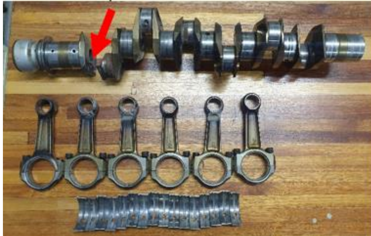
Photo 2: Fractured crankshaft assembly (digital).
