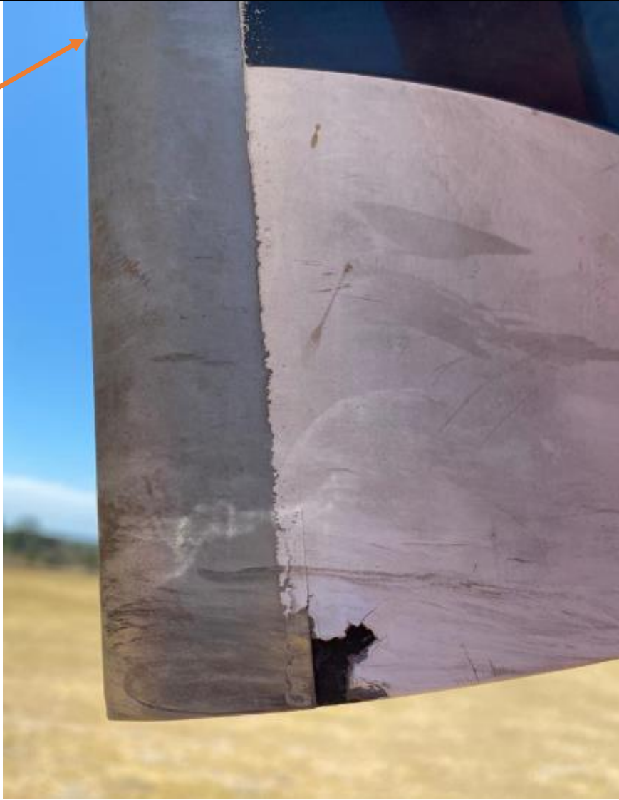
Figure 2: The damaged tail rotor blade with a nick on the leading edge. (Source: Operator)
