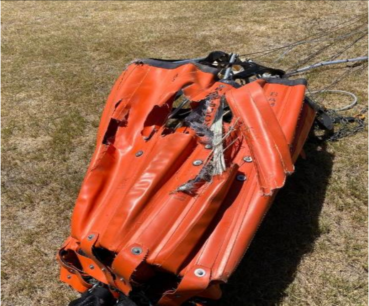
Figure 1: The damaged Bambi bucket. (Source: Operator)
