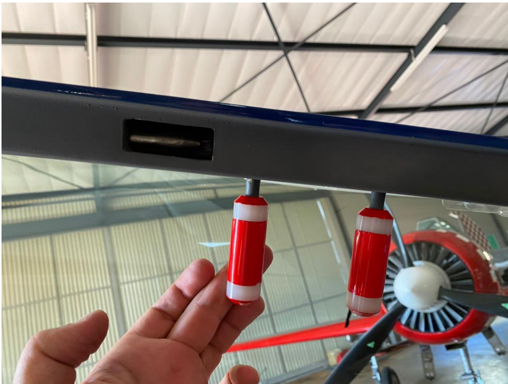
Figure 3: Latches of the canopy door on the aircraft. (Source: AME)
