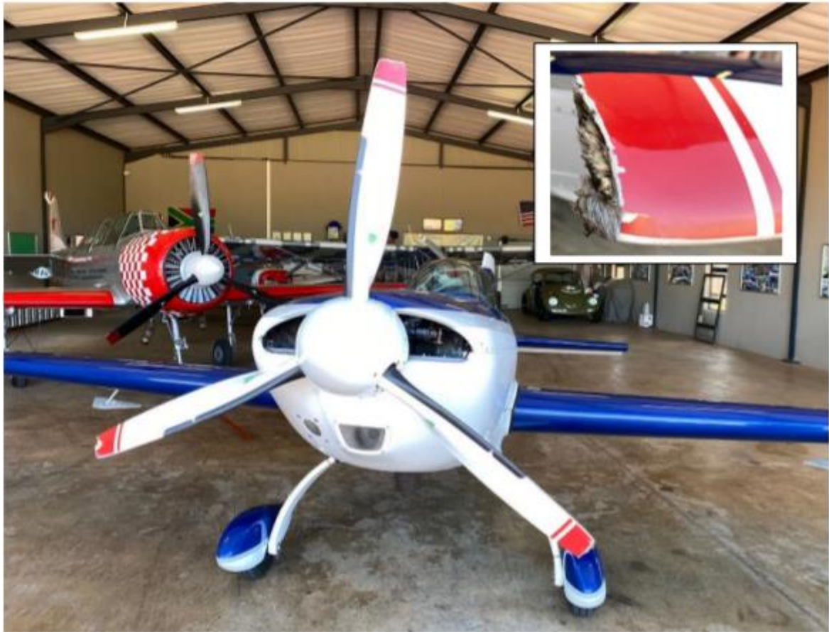
Figure 1: Damaged propeller blade tips. (Source: AME)
