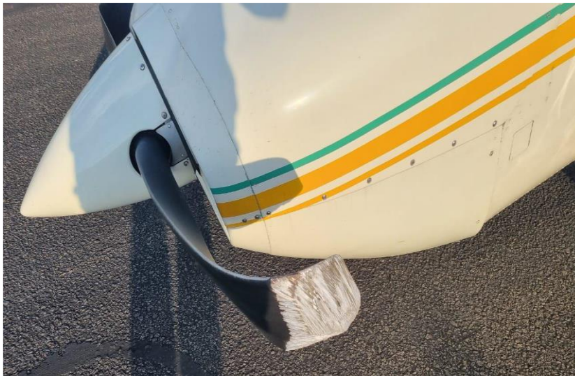
Figure 2: A bent propeller blade tip. (Source: Pilot)
