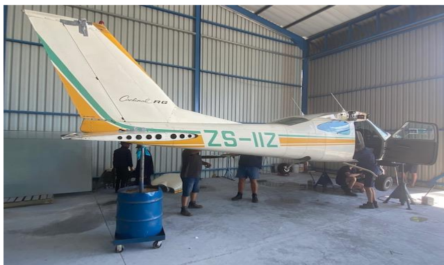
Figure 4: A view of the aircraft on jacks during the landing gear examination.
