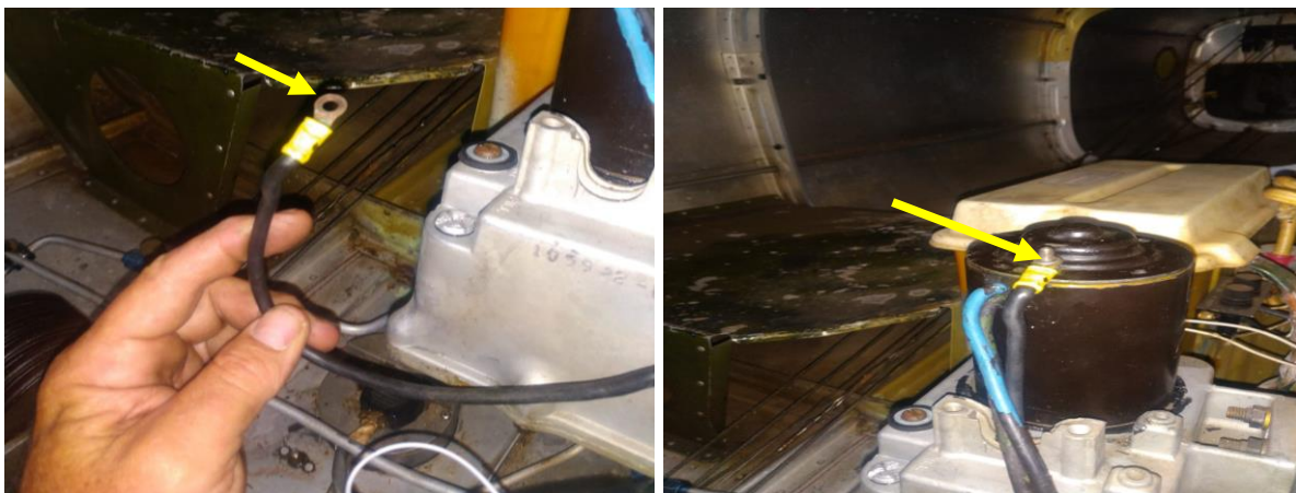
Figures 7 and 8: A disconnected gear pump motor cable (left picture); and a connected gear pump motor cable after maintenance (right picture).
