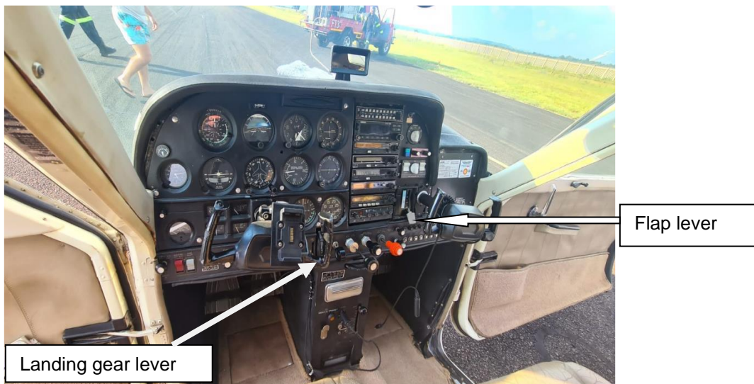
Figure 3: A view of the cockpit with the landing gear lever and flap lever in the down position.
