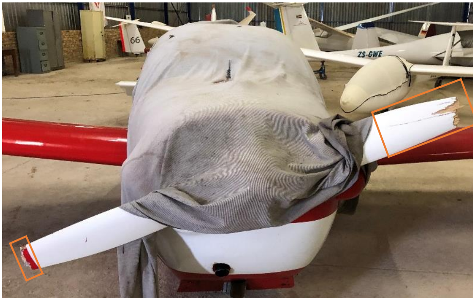
Figure 1: Damage to the propeller blades. (Source: Google Earth)
