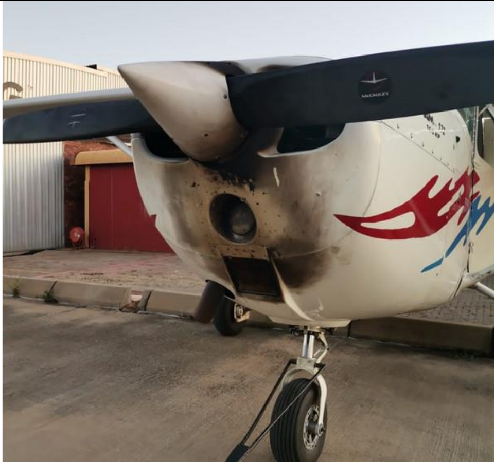
Figure 2: A close-up picture showing the black residue caused by the fire. (Source: Pilot)
